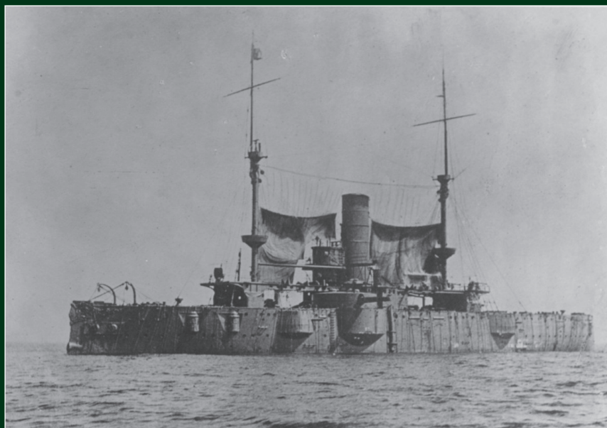
USS San Marcos prior to being fired upon by USS New Hampshire (BB-25) in ordnance tests in Chesapeake Bay, March 1911. Note that the old battleship has had canvas screens erected to increase her target area (photo: Naval History and Heritage Command).
